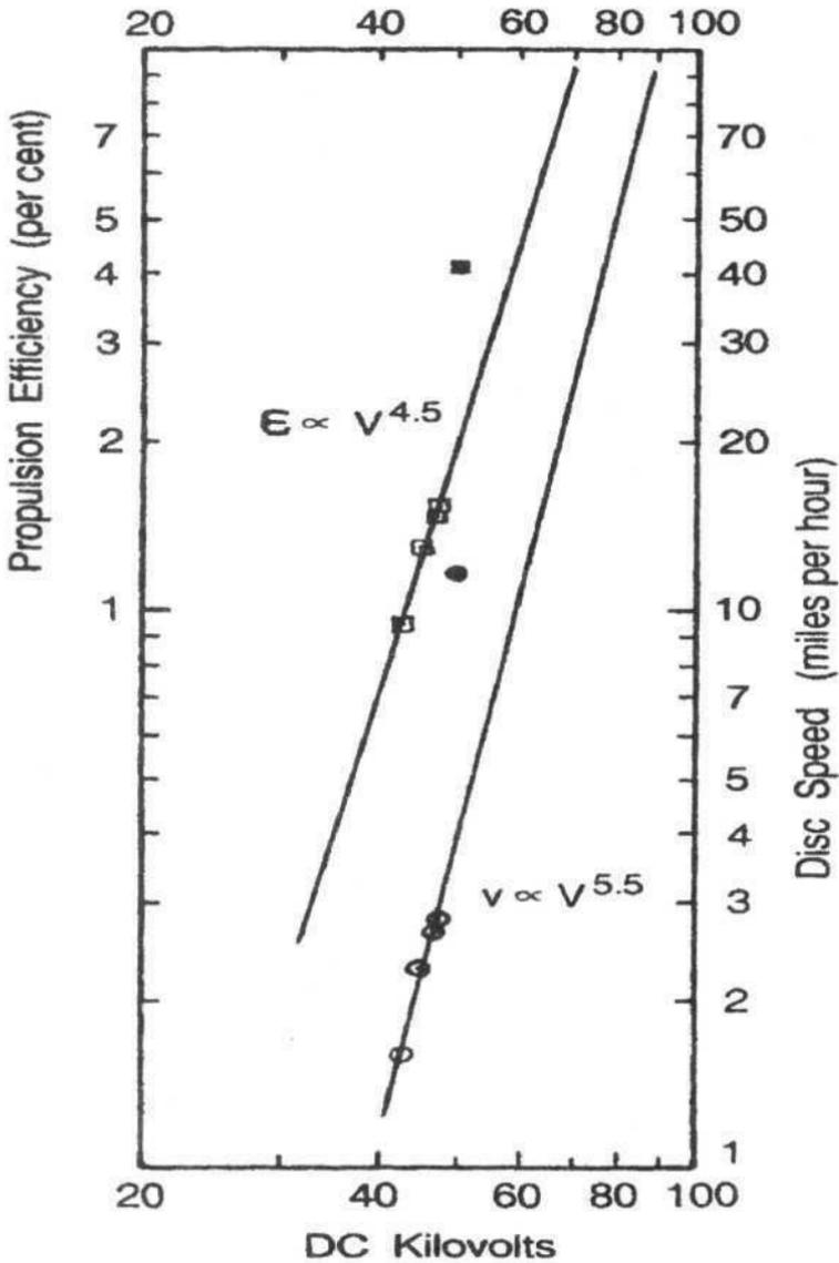
Disc speed  $v$  (□) and propulsion efficiency  $s$  (○) as a function of average DC voltage  $V$  plotted logarithmically from ONR test data. Filled points are data from a separate test carried out by T. T. Brown. (*Subquantum Kinetics*, LaViolette, p. 173)
