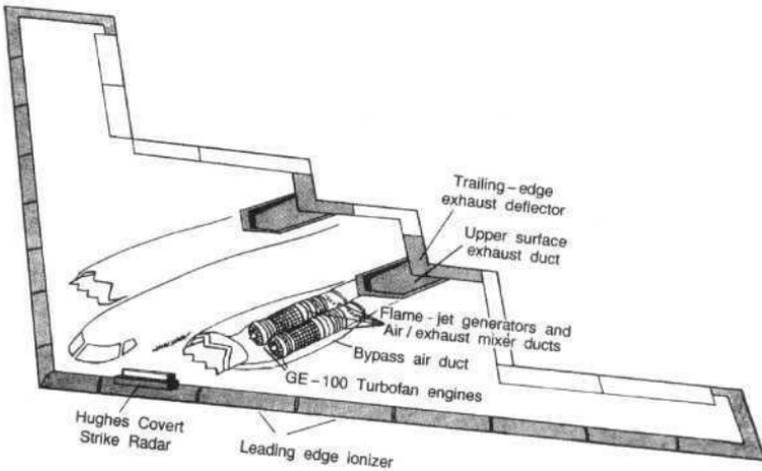
Figure 9. A view of the B-2 with a cutaway showing the arrangement of its flame-jet generators.
