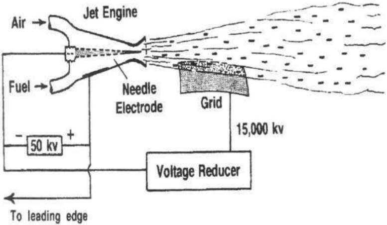
Figure 6. A high-voltage flame-jet generator.
