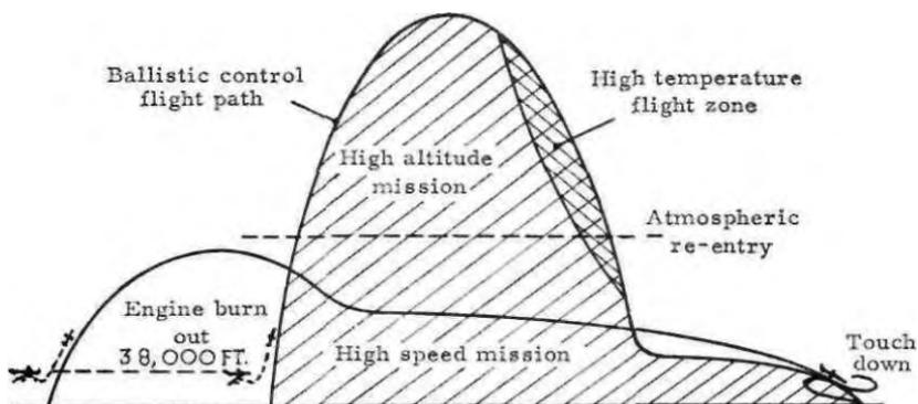
Fig 1. Basic flight programme of the X-15.
