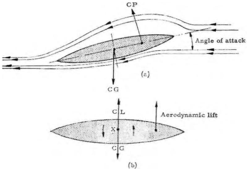
Fig 52. The Gyroscopic couples set up on an aerodynamically disturbed spinning disc.
