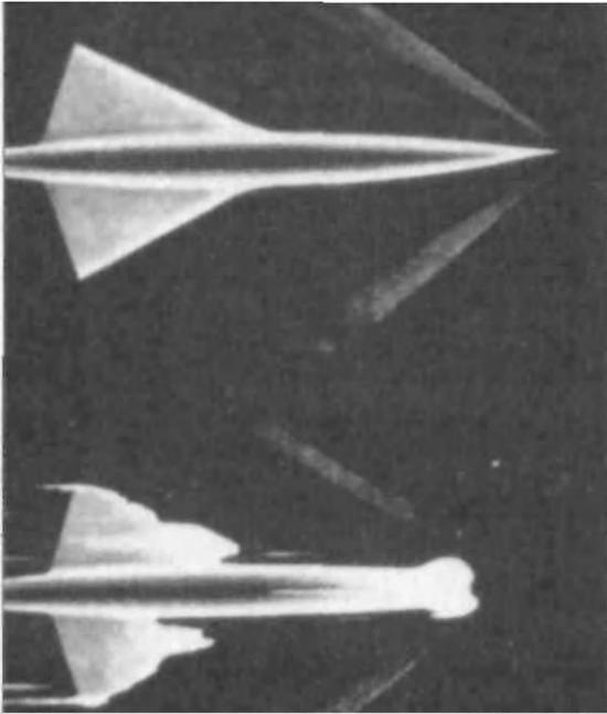
Plate 1. Stainless steel model subjected to air blast conditions likely to be met at five times the speed of sound. The temperature is about 3,000F.
