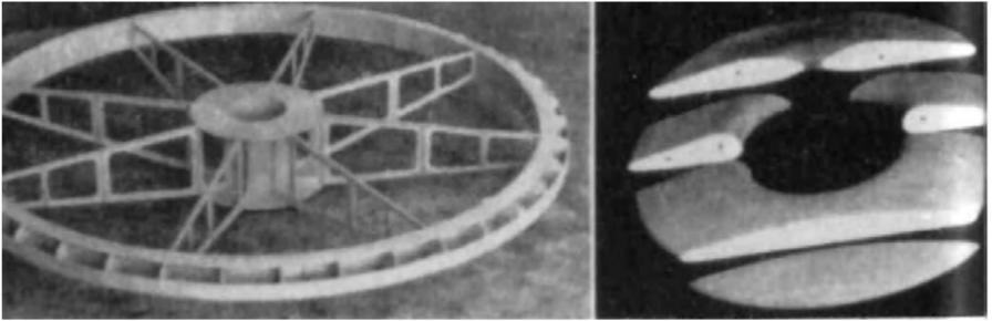
6ft dia. part structure illustrates simple construction of the circular wing.
