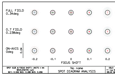
Fig. 6.6 Schmidt–Cassegrain with conic mirrors (focal surface radius: -380 mm; designed with Optisoft )
