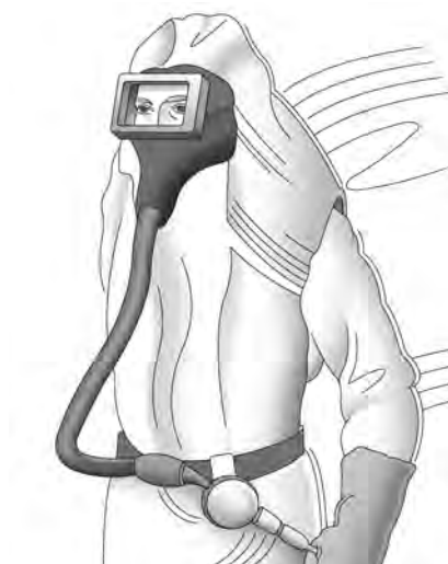
Full Facepiece Abrasive Blasting Continuous Flow APF=1,000 Needs to be fit tested
