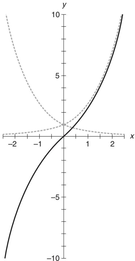
**Figure 14-5** Graph of the common exponential minus its reciprocal (solid black curve). The dashed gray curves are the graphs of the original functions.
