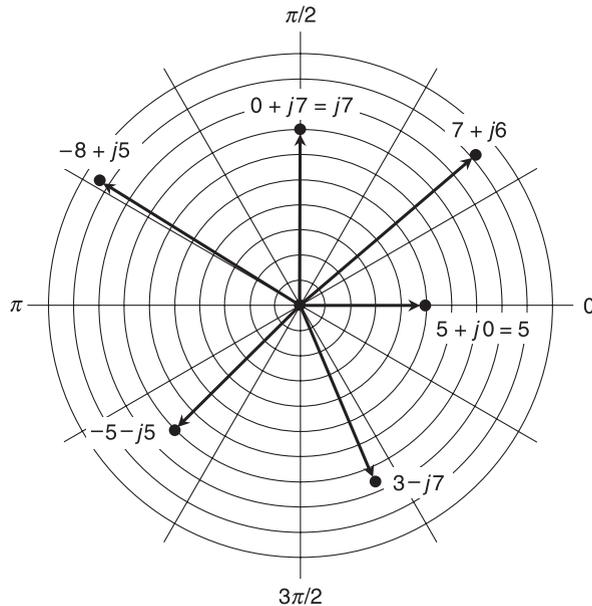
**Figure 6-5** Complex numbers can be portrayed as vectors in the polar plane. Each radial division represents 1 unit. Cartesian coordinates are shown here. The polar coordinates are entirely different!
