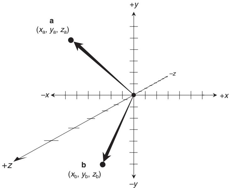
**Figure 8-1** Two vectors in Cartesian  $xyz$  space. This is a perspective drawing (as are all three-space renditions in this book). In “real life,” both vectors in this particular case would project generally toward us.
