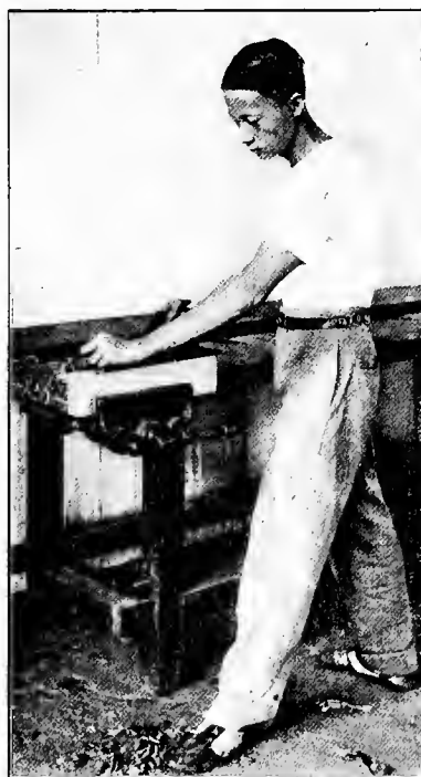
Fig. 109. Correct position for planing.
