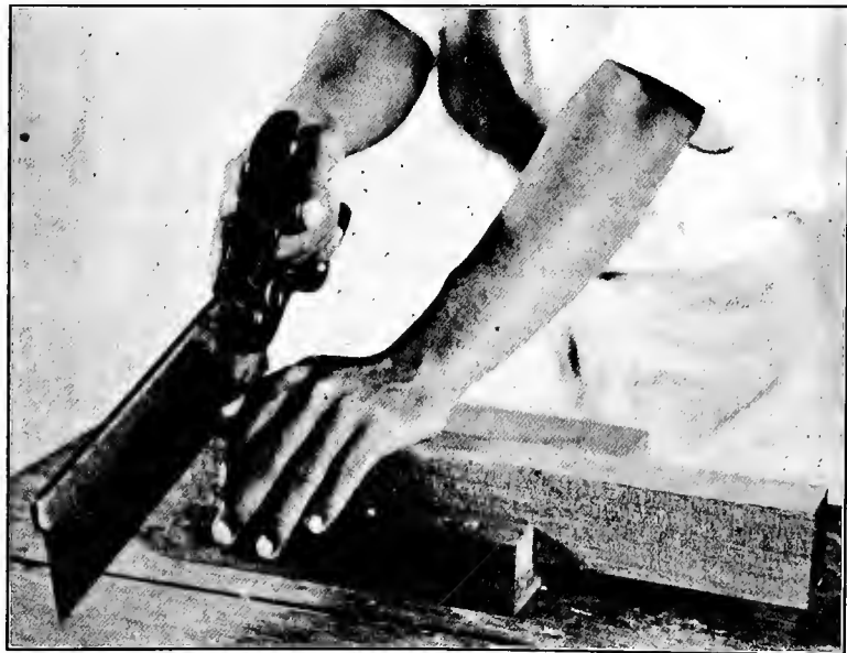
Fig. 114. Correct position in starting the backsaw.
