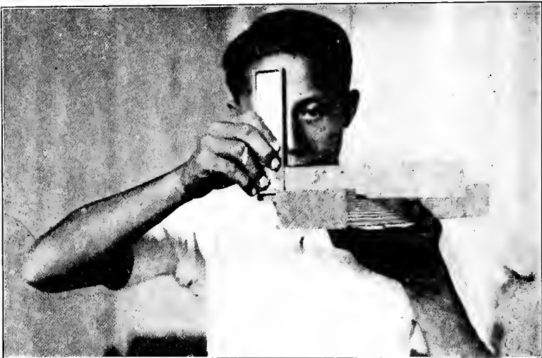
Fig. 119. Testing a finished cut.
