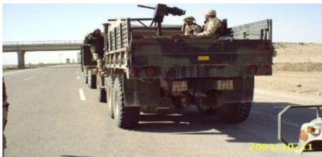
Figure 6-4. Armor Plating Surrounding the Gun Platform
