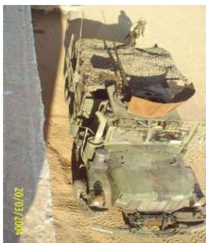
Figure 6-6. Gunner's Shield and Camouflage for the Bed of the Truck
