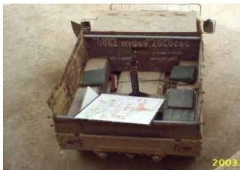
Figure 6-5. Armor Plating Surrounding the Gun Platform (Also on Bed of the Truck)
