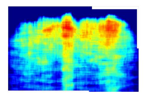
Analysis of the structures above Belzoni's chamber: intensely colored spots can be observed, appearing in all tomographic images taken from different angles, corresponding to internal artificial structures.
