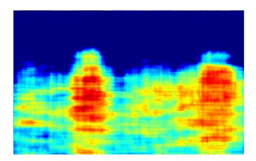
Improvement of the signal-to-noise ratio revealing the internal structure of the 5 Zeds, consisting of 5 horizontal levels and a sloping roof
