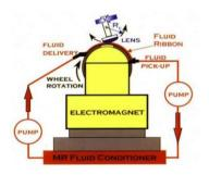
Fig. 11: Polishing Device using MR Fluid
