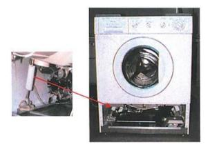
Fig.8: MR Fluid dampers in Washing Machine
