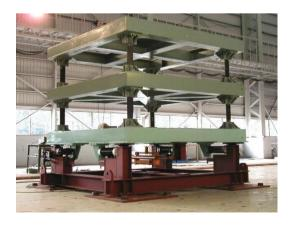
Fig. 6: A MR Seismic Damper Test sample
