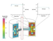
**Fig. 10:** MR Fluid-based brake
