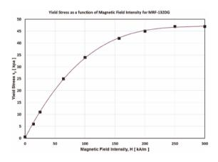
Fig. 3: Yield stress as a function the magnetic field strength
