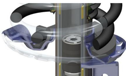
**Fig. 5:** MR Fluid dampers in Seat Suspension
