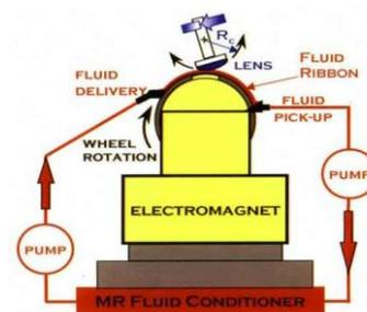
Fig. 11: Polishing Device using MR Fluid
