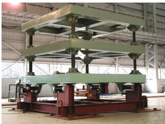
**Fig. 6:** A MR Seismic Damper Test sample
