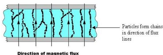
**Fig. 2:** MR Fluid in presence of Magnetic Field
