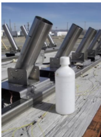
Simulator Projectile Airburst Liquid (SPAL) system
