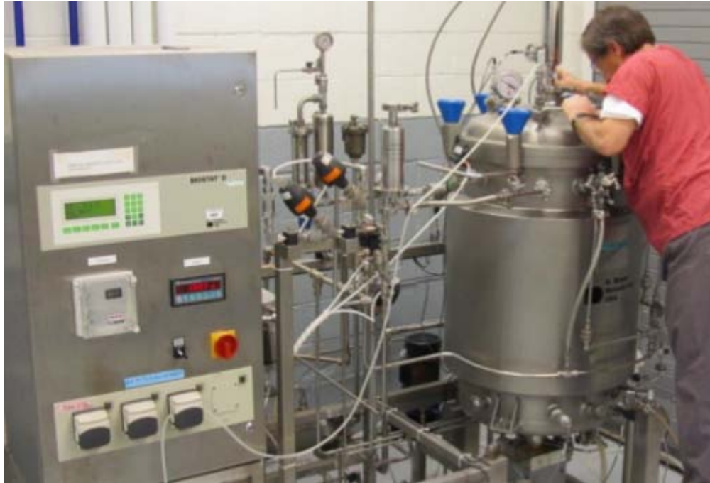
A large 1500 L fermentator. Photos credit: Dugway Proving Ground
