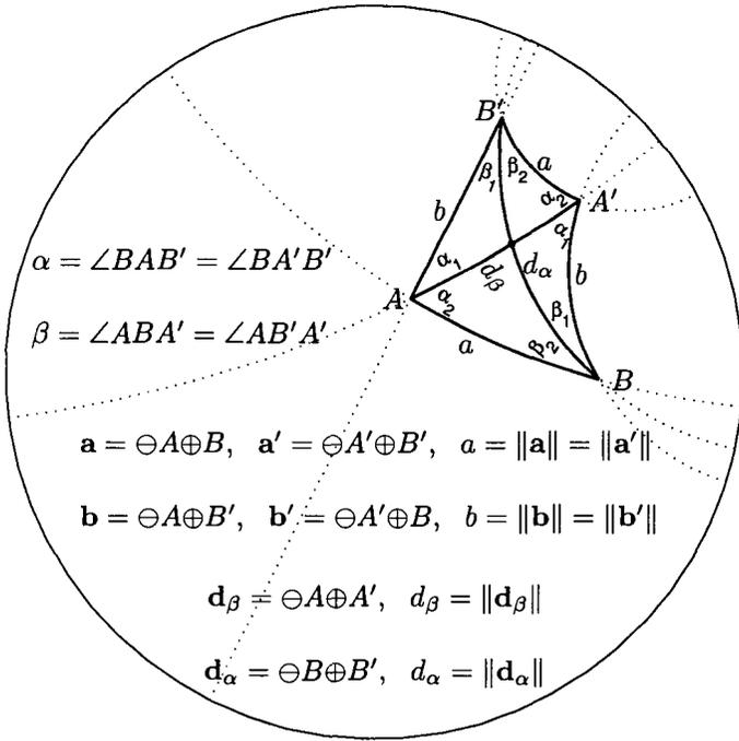
Fig. 8.23 Gyrotriangle defects in the Möbius gyroparallelogram in the Möbius gyrovector plane  $(\mathbb{R}_{s=1}^2, \oplus, \otimes)$ . The gyroparallelogram  $ABA'B'$  has (i) two side gyrolengths,  $a$  and  $b$ ; opposite sides are congruent; (ii) two gyroangles,  $\alpha$  and  $\beta$ ; opposite gyroangles are congruent; and (iii) two diagonals,  $d_\alpha$  and  $d_\beta$ . The diagonals concurrent point coincides with their gyromidpoints. Alternate gyroangles are congruent.
