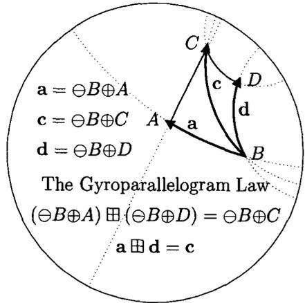
Fig. 8.21 The gyroparallelogram law and the Möbius gyroparallelogram  $ABDC$  in Fig. 8.19 give rise to the commutative gyroparallelogram addition law of gyrovectors, shown here as a first example.
