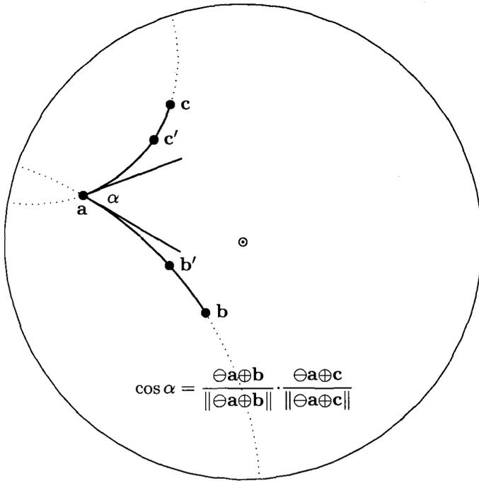
Fig. 8.1 A Möbius gyroangle  $\alpha$  generated by two intersecting Möbius geodesic rays (gyrorays). Its measure equals the measure of the Euclidean angle generated by corresponding intersecting tangent lines.
