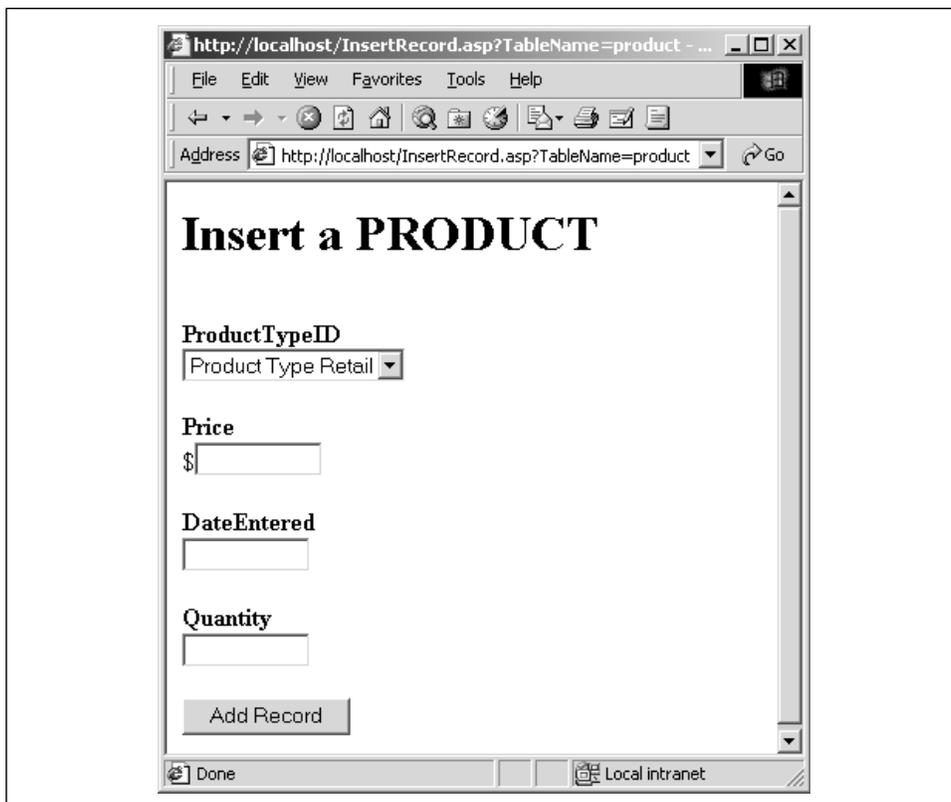
Figure 6-9. The “Insert a New Record” administration page for the *Product* table permits the user to create a new record
