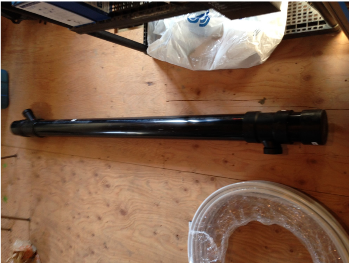
This shows the new 4 inch ABS pipe section and the coil of PEX that will be used to make the drain water heat exchanger..
