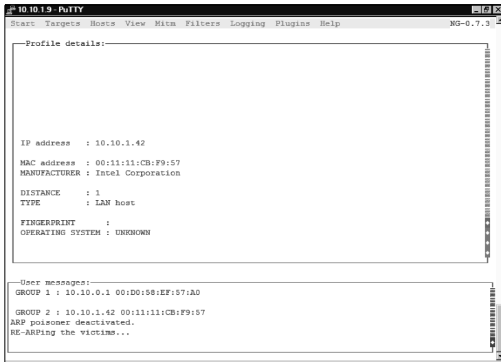
Figure 6.8 Ettercap Successfully Restoring the Mangled ARP Tables
