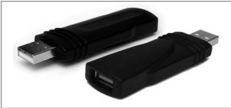
Figure 9.2 KeyGhost with USB Connectors
