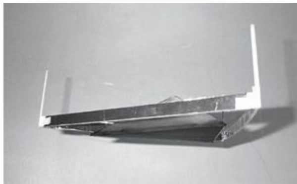
Figure 12.12. A lifter built and tested by Jean-Louis Naudin. (Photo courtesy of J.-L. Naudin, from his website, http://jnaudin.free.fr/ )
