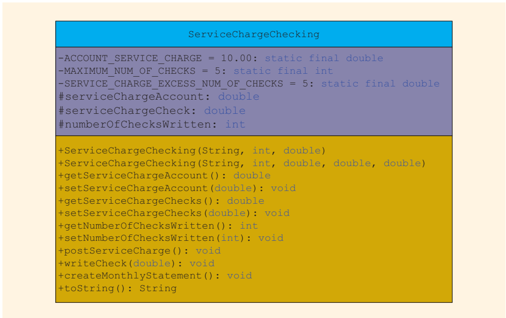
FIGURE 10-10 UML class diagram of the class ServiceChargeChecking
