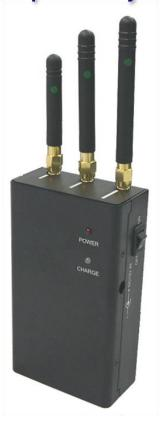
Capable of jamming the frequency bands assigned to UMTS/HSPA in a particular location, while leaving the GSM/GPRS/EDGE bands undisturbed
