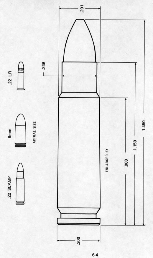
Figure 6-2. .22 Caliber SCAMP Cartridge.
