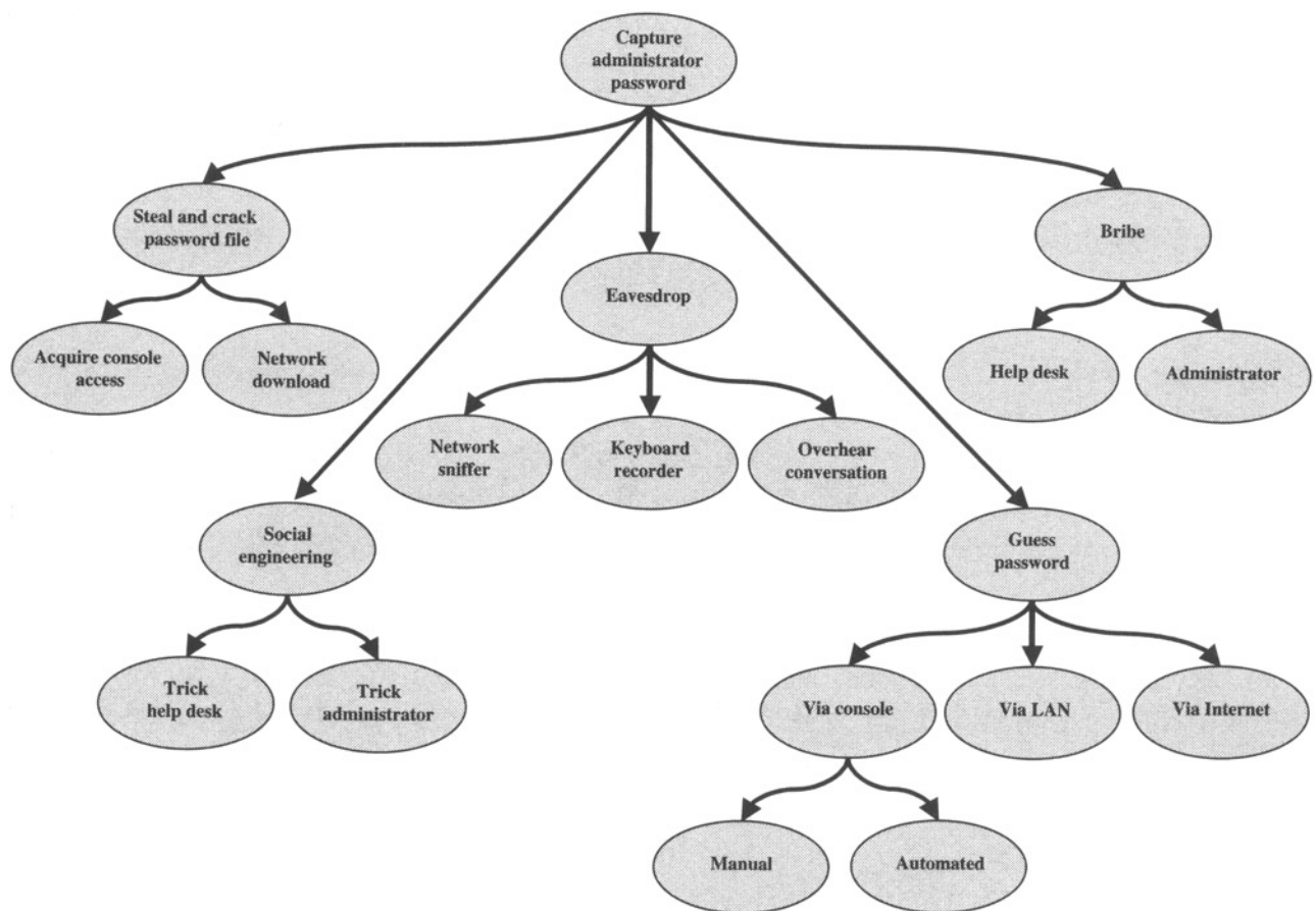
Figure 10.1: Fault tree example.
