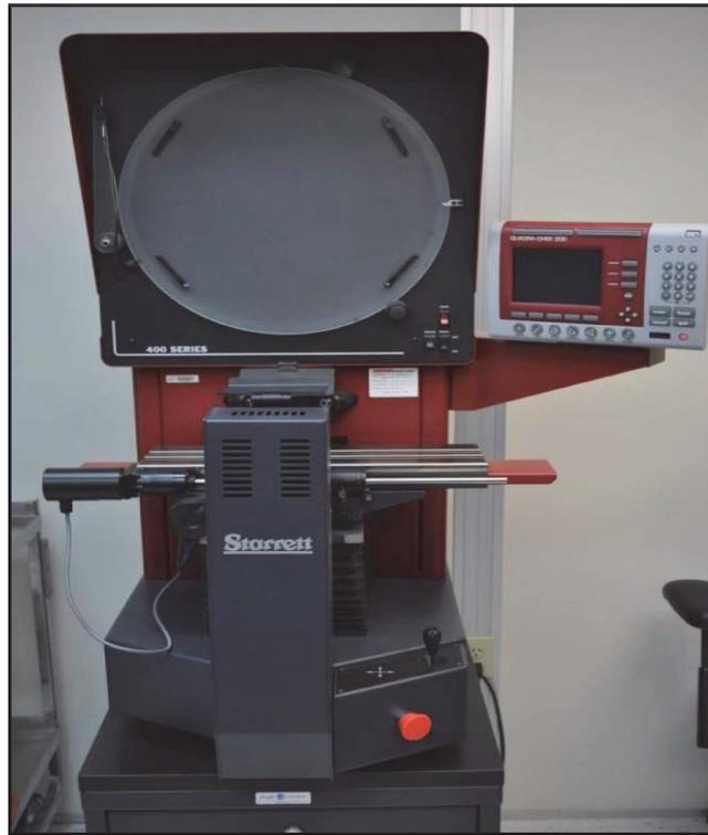
**Figure 2-16.** NIOSH Optical Thread Comparator
