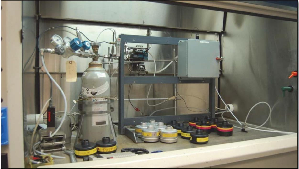
Figure 2-8. NIOSH Service Life Test Chamber
