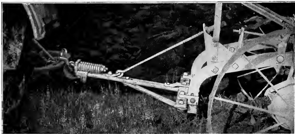
Illust. 8. Showing proper hitch for 2-bottom plow
