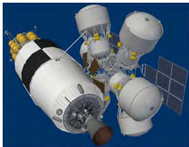
Figure 5.2.1-2. Artist's concept of a fuel depot servicing an Earth Departure Stage. Source: Boeing
