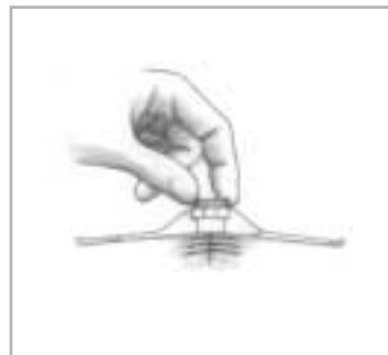
3. To adjust tension, lift capstan.
