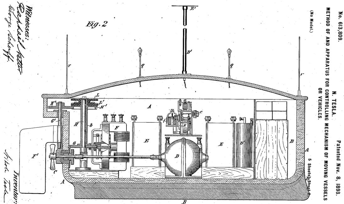
Figure 9 Tesla's Telautomaton patent. (See Image Note 9)
