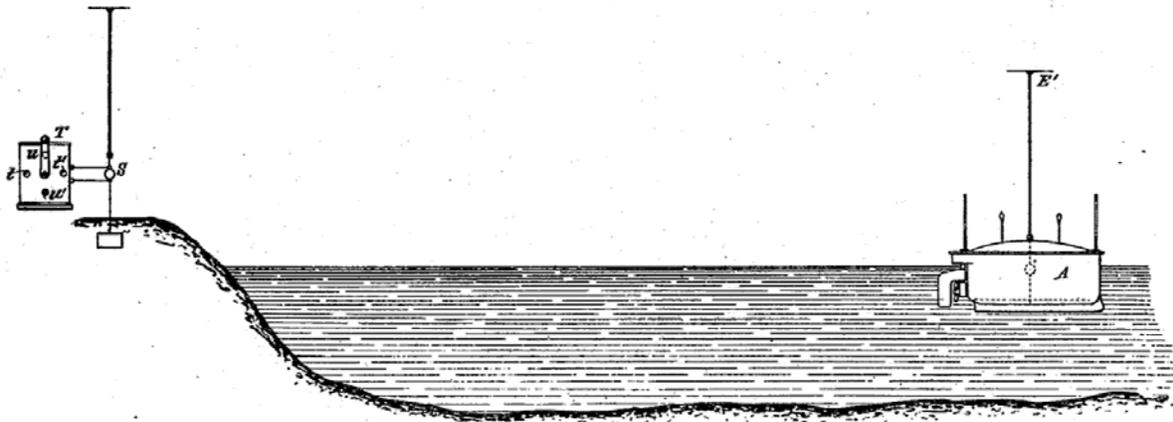
**Figure 11** Image from Tesla's patent of the telautomaton showing the transmitter and telautomaton in operation (See Image Note 11).
