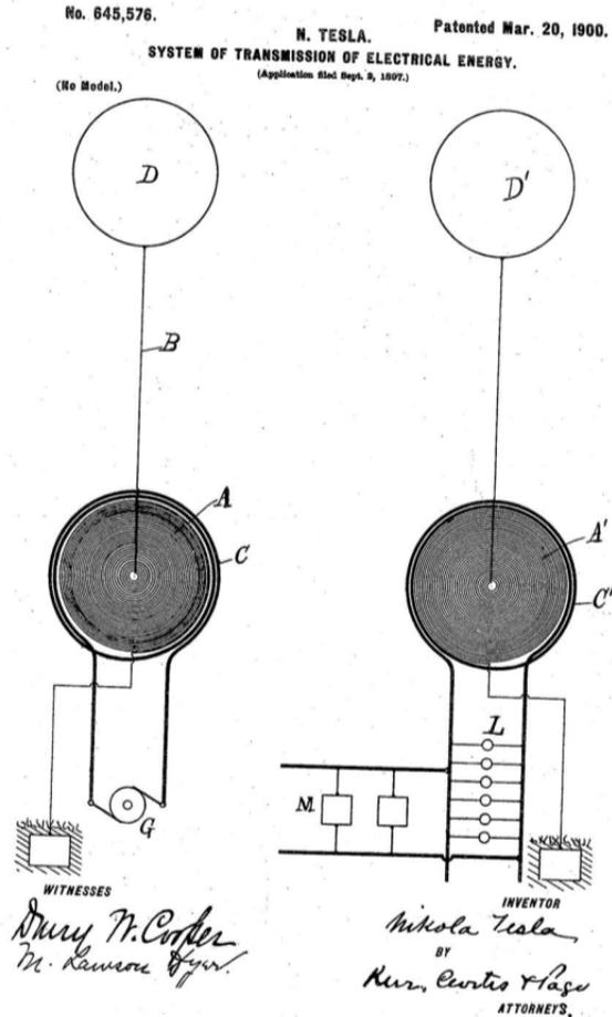
**Figure 7** Tesla's patent for a system of wireless energy transmission. (See Image Note 7)
