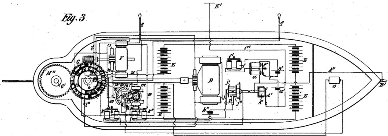
Figure 10 Top down diagram of the telautomaton’s internal circuitry. (See Image Note 10).
