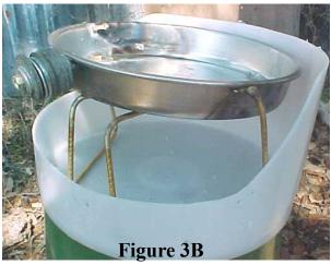
bottom of the distribution pan. The pans we were using fit with about 1/2 inch of space around the lip when put in the bottom of a plastic 5 gallon bucket as seen in Figure **3B**. This worked well for years but there was a simpler way.
